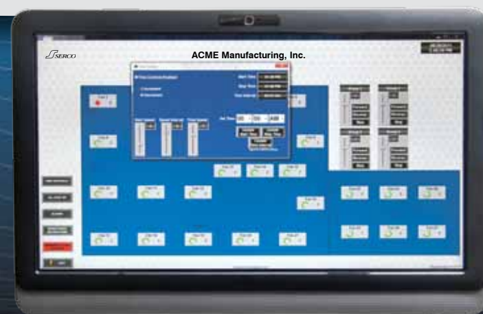
Timer setting dialog box enables direction and speed for individual fan or zones to be set by time of day. A similar dialog box is available based upon temperature settings.
